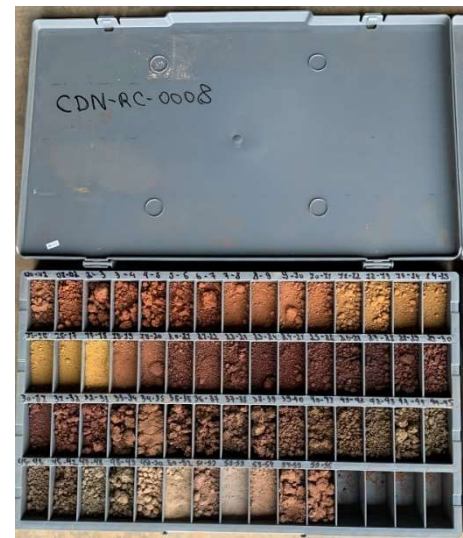
Figure 4: CDN-RC-0008 drill cuttings which has been reported as having 31 m intercept @11.2% \text{TiO}_2 including 10 m intercept @14.8% \text{TiO}_2
