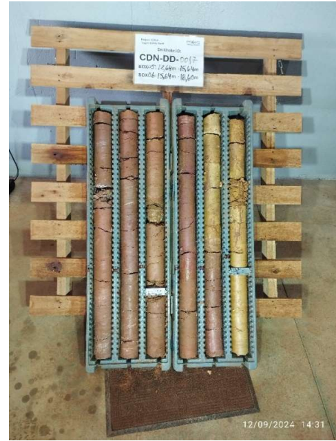
Figure 2: CDN-DD-0017 drill core which has been reported as having 16.4 m intercept @13.1% \text{TiO}_2 including 5 m intercept @16.3% \text{TiO}_2
