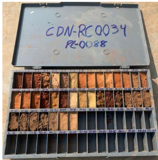
Figure 3: CDN-RC-0034 drill cuttings which has been reported as having 34 m intercept @10.0% \text{TiO}_2 including 9 m intercept @17% \text{TiO}_2
