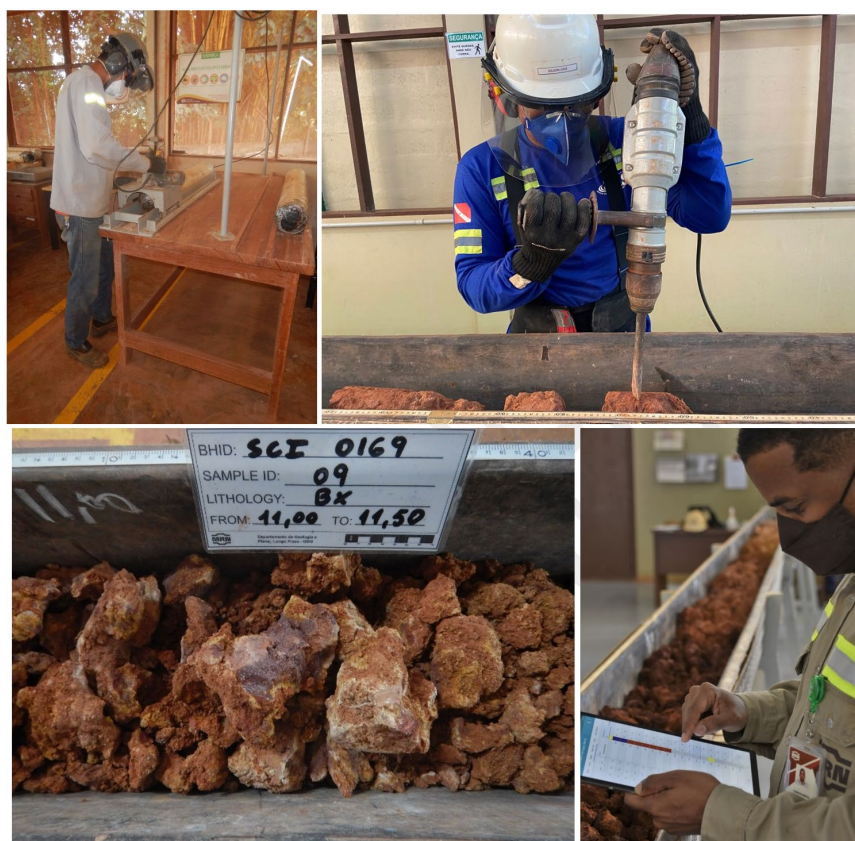
Figure 26 Photographic documentation of the core sample cover removal, crumbling, intervals splitting and logging
