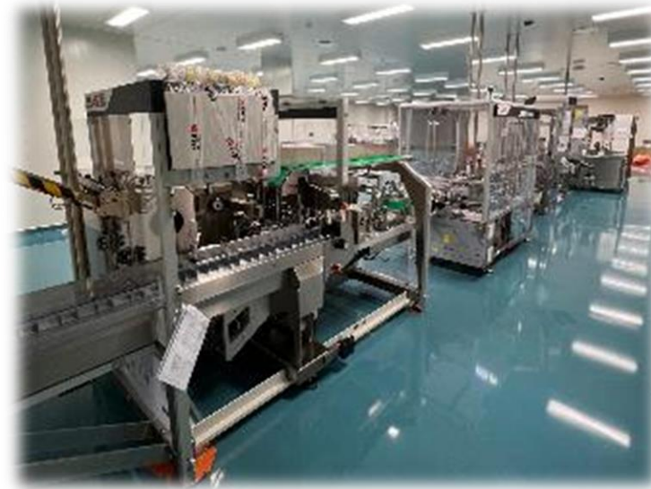
Packaging Hall - Cartoner, Tamper Evident Labeller, Bundler & Case Packer
