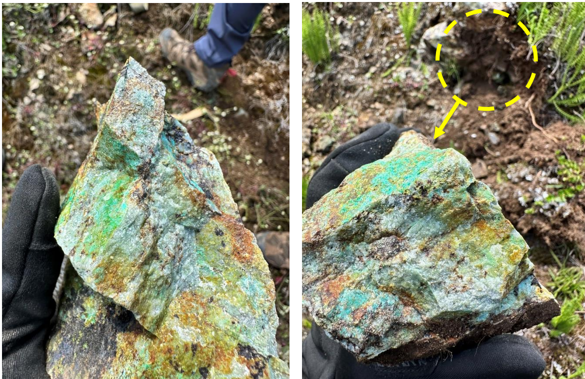
Figure 4: Copper outcrop within Irka-Sur discovered under soil cover hosting chalcopyrite veining, malachite and copper oxides.
