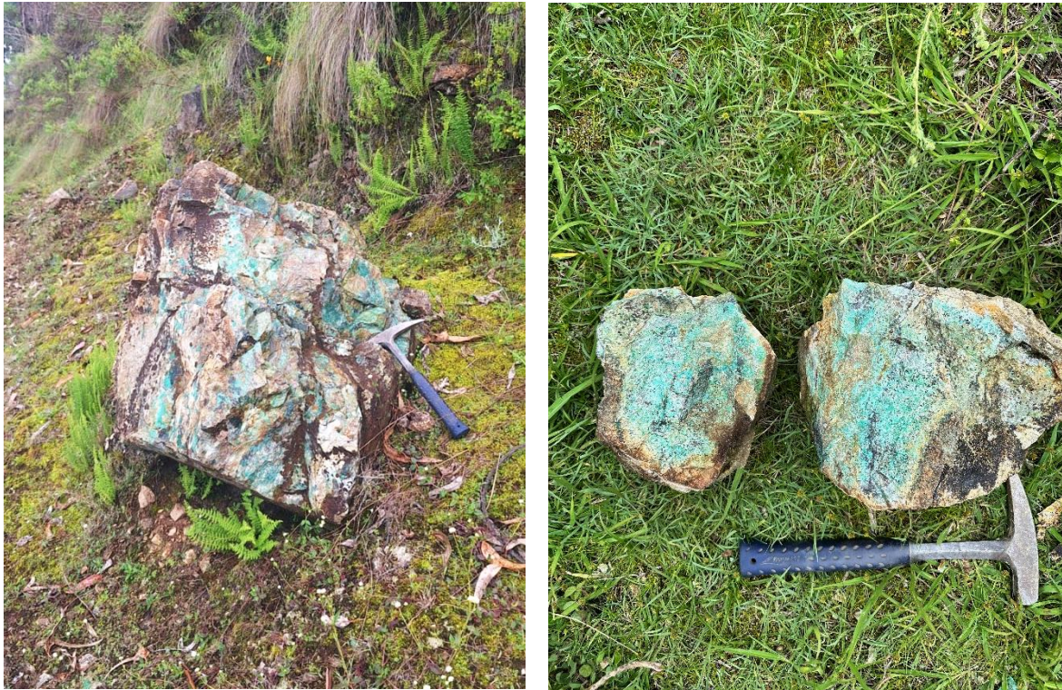
Figure 3: Left – Large outcropping boulder of significant copper bearing Malachite mineralisation similar to the discovery outcrop found on Haquira in 2001, located along strike Venatica on the same Andahuaylas-Yauri belt, with Quartz, Malachite, Fe-Ox, later taken over by First Quantum for CAD $650M 6 . Right – Float boulder with significant visual copper, found on the highest level prospected of the Irka Sur hill, which indicates system continues extending higher.
