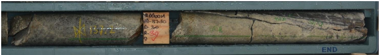
Figure 5 – Drill core photo from TRDD001A showing sulphide veining at 137m downhole.
