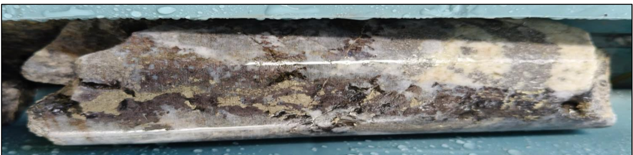
Figure 1 – Sulphide Vein from TRDD001A (HQ core size) showing sulphides within quartz and carbonate veining.
