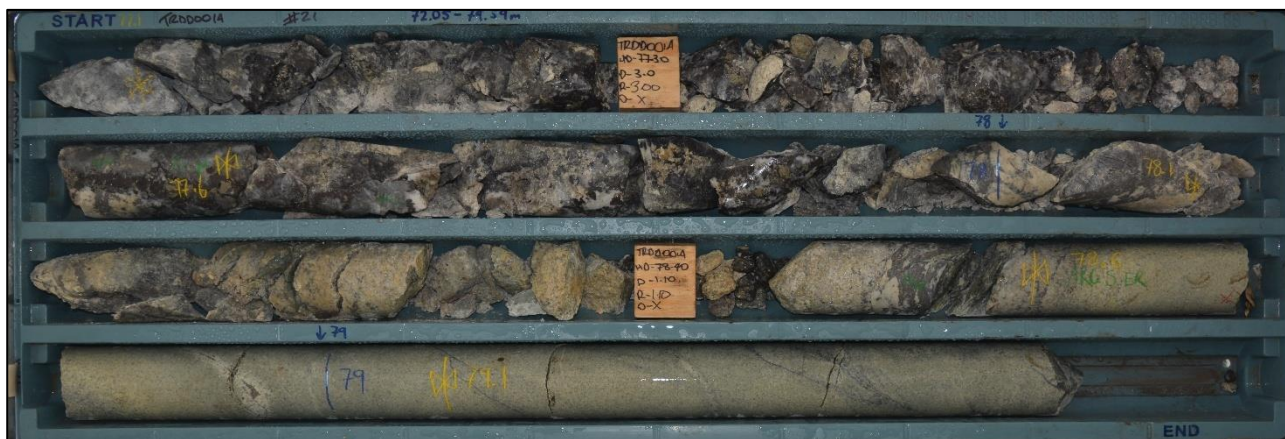
Figure 4 – Drill core photo of tray 21 from TRDD001A showing core between 77.05m and 79.1m.
