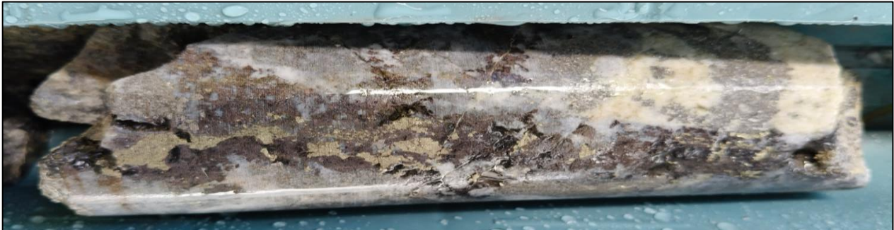
Figure 1 – Sulphide Vein from TRDD001A (HQ core size) showing sulphides within quartz and carbonate veining, included in sampling from 77.1 to 77.6m
