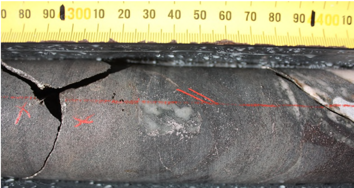
Figure 6. RD045 406.2 – 406.3. fine grained arsenopyrite intergrowth around silica within disseminated pyrrhotite groundmass. 1
