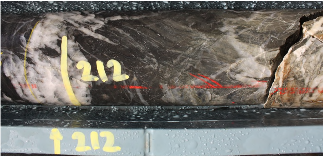
Figure 4. RD045. 212.00 212.20m Acicular arsenopyrite needles developed adjacent to steeply inclined shear structure within overlying western sediments. 1
