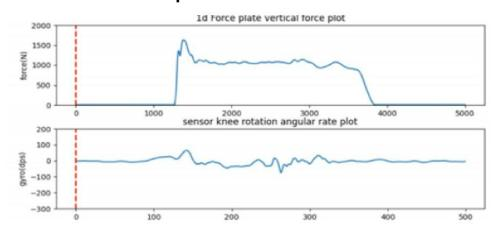
The second graph (Graph.2) shows data for **Poor landing** in which the tibia rotates at 230 °/sec (approx. 25°) which is detected by the 3D sensor yet not by the 1D force plate. This rotation is an element that potentially stresses the Anterior Cruciate Ligament (ACL) causing adverse tension and increasing the risk of injury.
