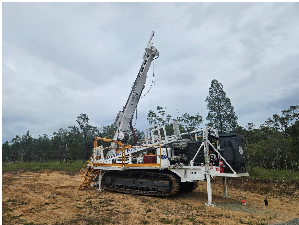
Figure 1 Track-mounted reverse circulation (RC) drill rig at Orient West
