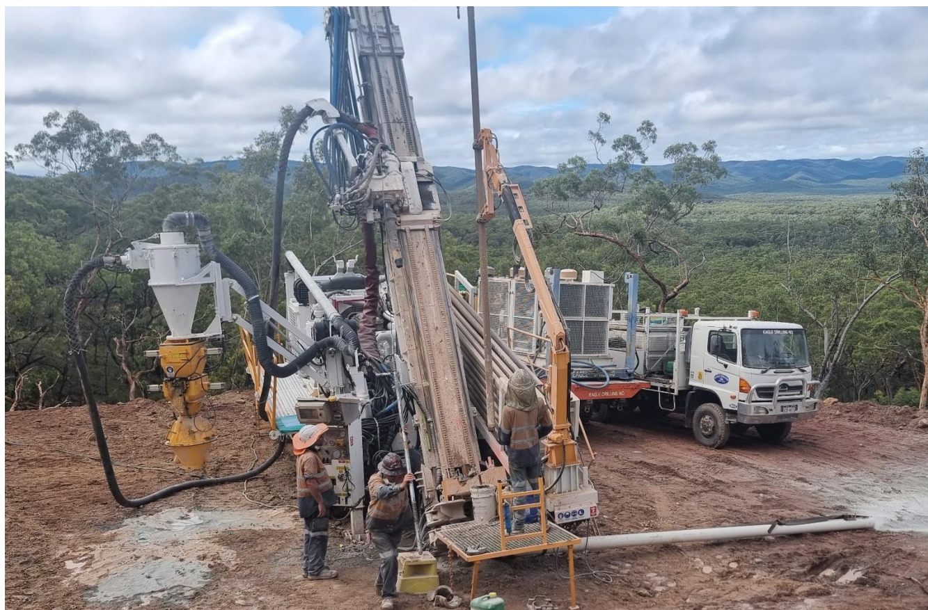
Figure 1 Track-mounted reverse circulation (RC) drill rig at Orient West (ORR069)
