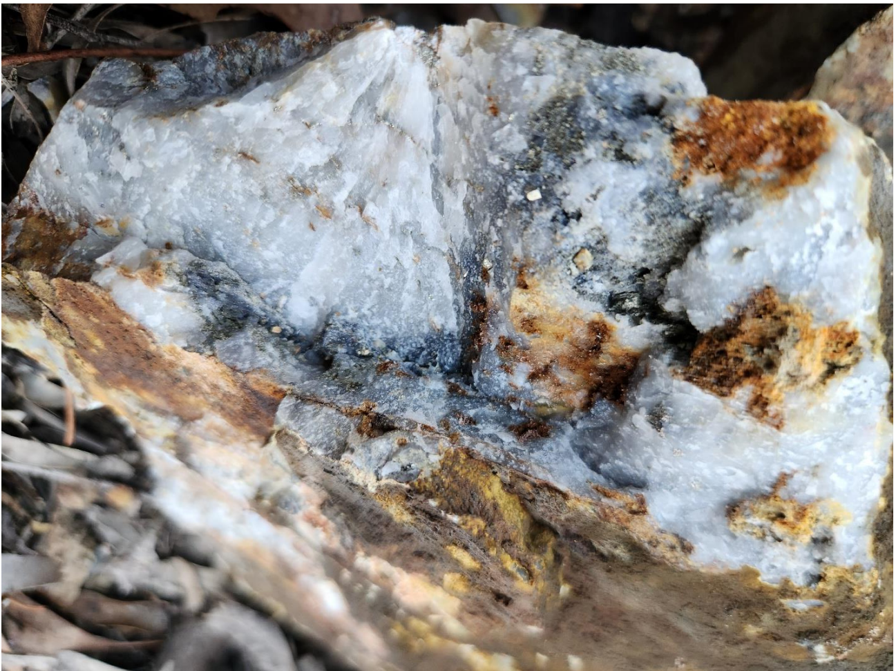
Figure 2: Sulphides in quartz from sample DRC006, abundant pyrite and arsenopyrite. Small quantities of stibnite (0.2%) was tentatively identified and is subject to confirmation by assay.
