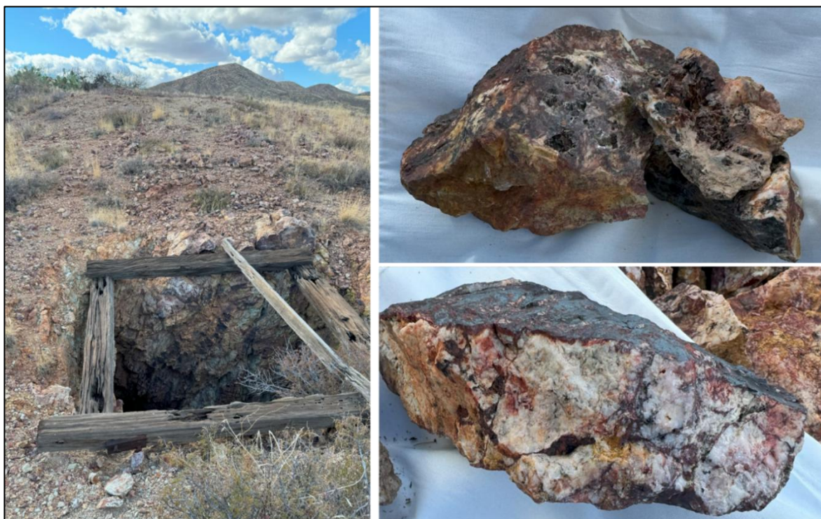
Figure 1: Aurora historic shaft, with high grade gold assays from samples of 10.8 g/t Au, and 9.83 g/t Au.
