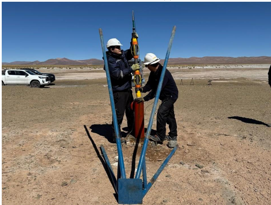
Figure 1. Permanent magnet and antenna are lowered into a borehole to record the response of the nuclear magnetisation associated with hydrogen nuclei in the pore fluids (eg. groundwater) of the formation.
