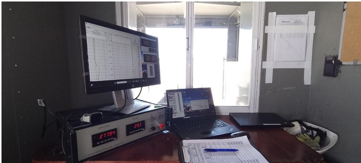
Figure 2. Checking that the NMR gamma, resistivity, porosity, temperature data has been collected.
