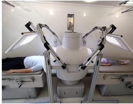
Orion LifeSpan™ configured for hyperscanning. Father and daughter subjects are measured simultaneously to study interactions. Synchronisation of the sensors in the two helmets is within 1 msec. Pic: Compumedics
