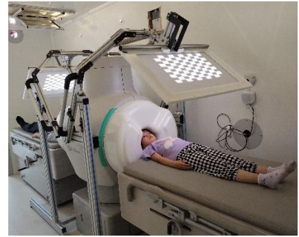
Orion LifeSpan™ configured for hyperscanning. Father and daughter subjects are measured simultaneously to study interactions. Synchronisation of the sensors in the two helmets is within 1 msec. Pic: Compumedics
