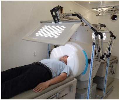
Orion LifeSpan™ configured for hyperscanning. Father and daughter subjects are measured simultaneously to study interactions. Synchronisation of the sensors in the two helmets is within 1 msec. Pic: Compumedics
