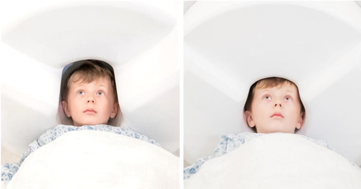
Five-year-old child in an adult sized MEG helmet (left) and the same child in a helmet optimised for paediatric measurements (right). Pic: Compumedics
