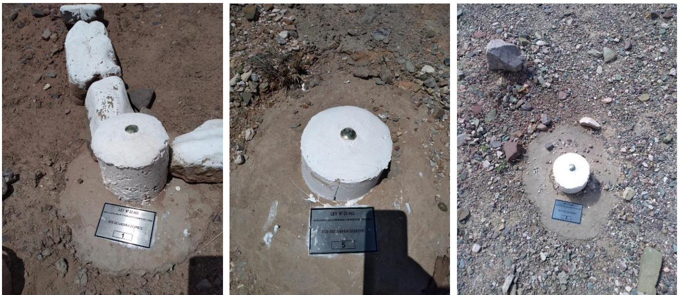
Figure 3. Survey points established on each corner of the concessions.
