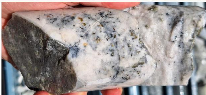
SDDSC161 intercept: 0.2 m @ 4,700 g/t Au and 0.25% Sb from 511.3 m showing abundant visible gold in a quartz-carbonate-stibnite vein. Part of a wider zone grading 3.4 m @ 466.4 g/t AuEq (466.0 g/t Au, 0.2% Sb) from 508.4 m. Core diameter is 63.5 mm.
