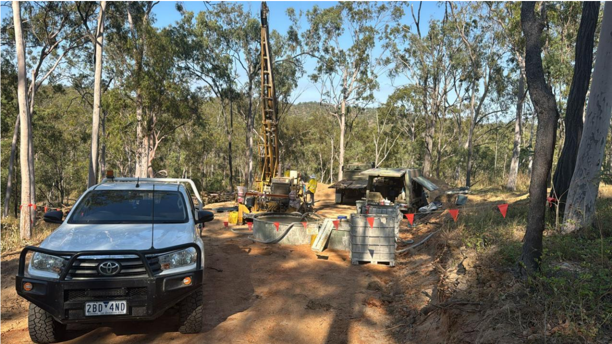
Figure 2: Diamond core drill site setup at New Constitution.
