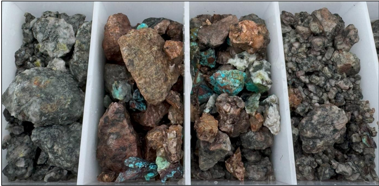
Figure 3: Copper carbonate mineralisation within an oxidised structure in PRC006 (120ft to 128 ft)
