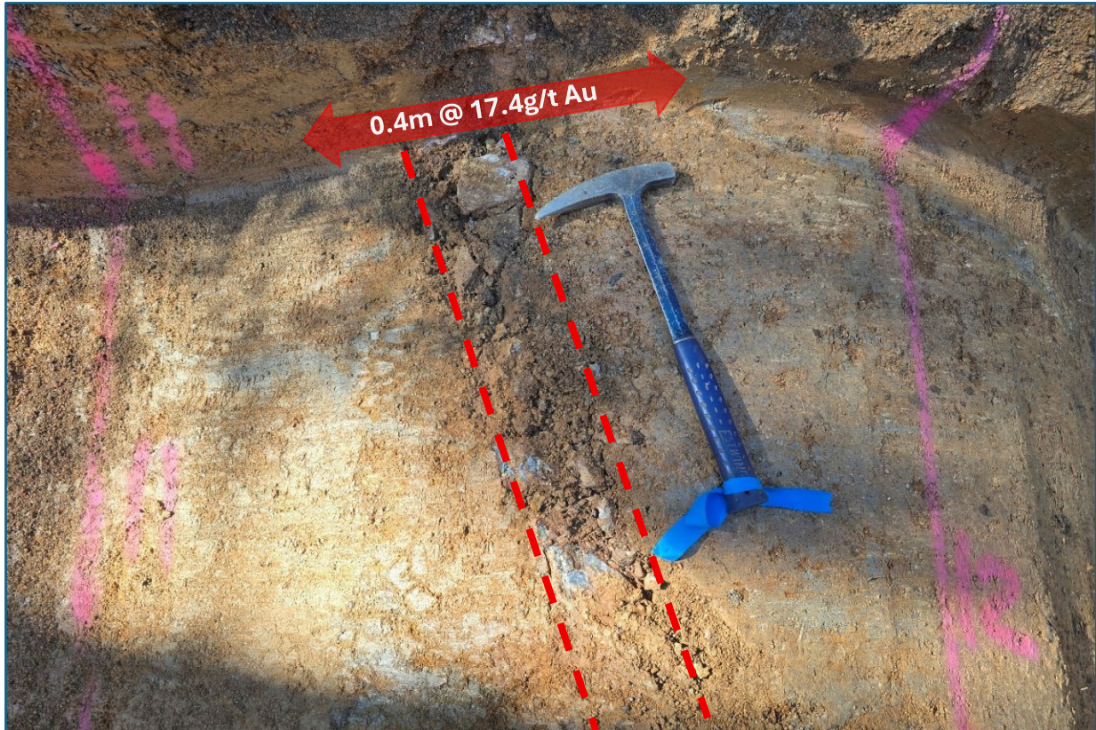
Figure 4 – Trench 6 (11-12m Interval) showing discrete quartz/arsenopyrite/pyrite rich vein between red dashed lines (11.3-11.7m interval including the vein graded 0.4m @ 17.4g/t Au).
