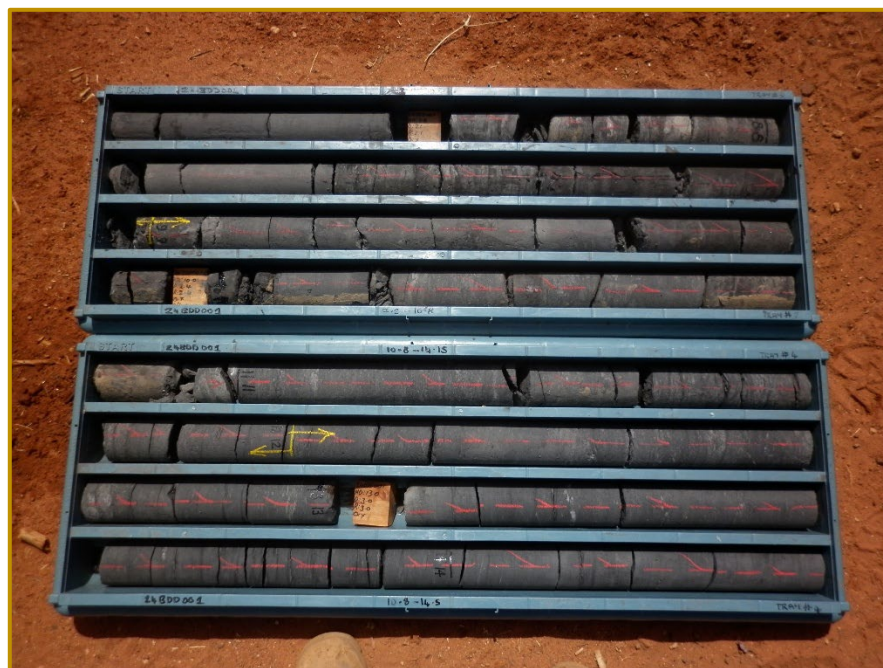
Figure 2. Byro Core Tray (Drillhole 24BDD002 Depth 7.2 – 14.15m), showing Permian black Shale from shallow depth (refer ASX announcement 25 February 2025)
