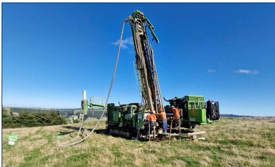
Figure 11: Photo of RC drilling operation on Waipori Station (EP60807 - Lammerlaw)
