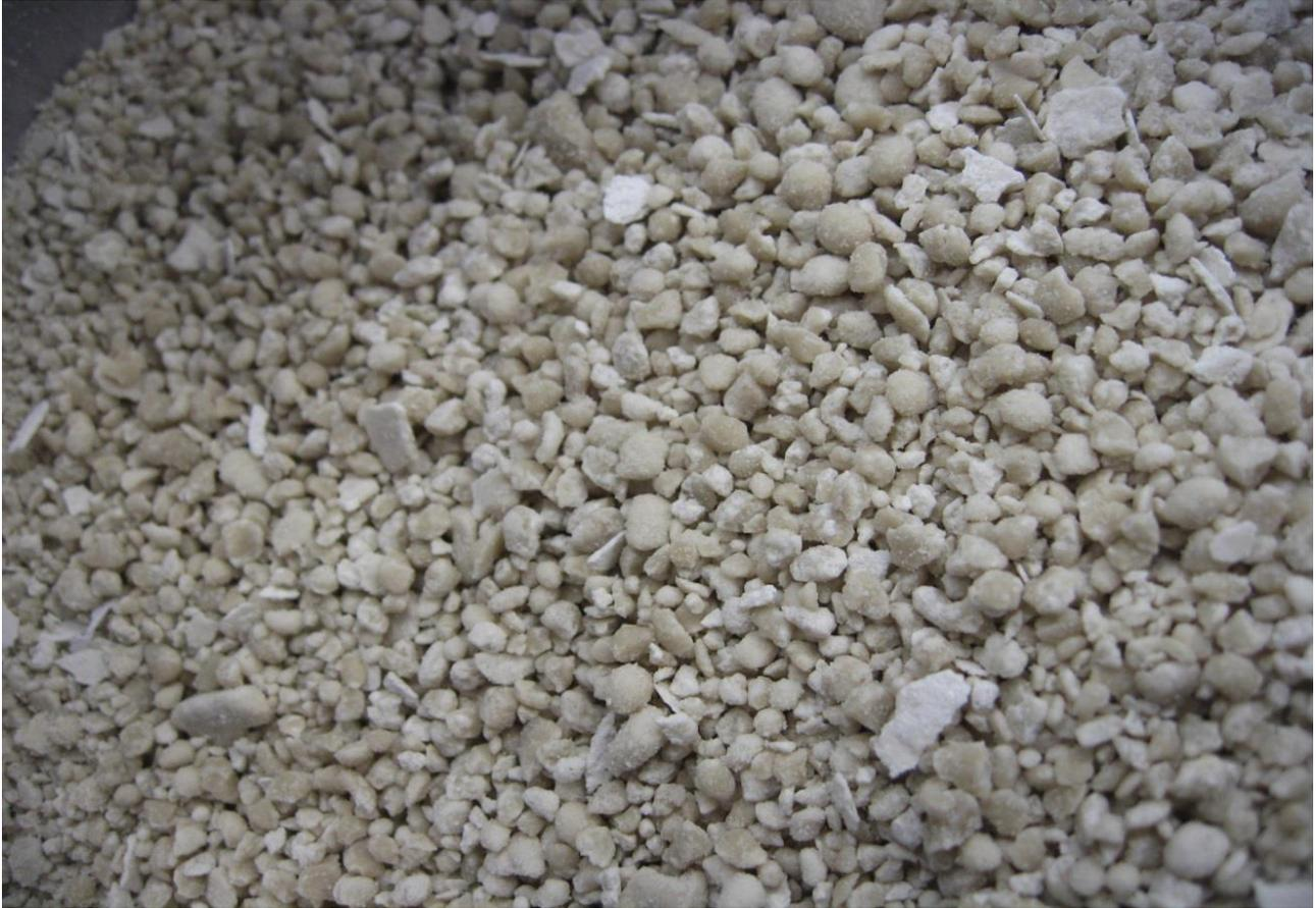
**Di Ammonium Phosphate fertiliser produced from Ammaroo Phosphate Rock at Prayon's laboratory in Belgium**
