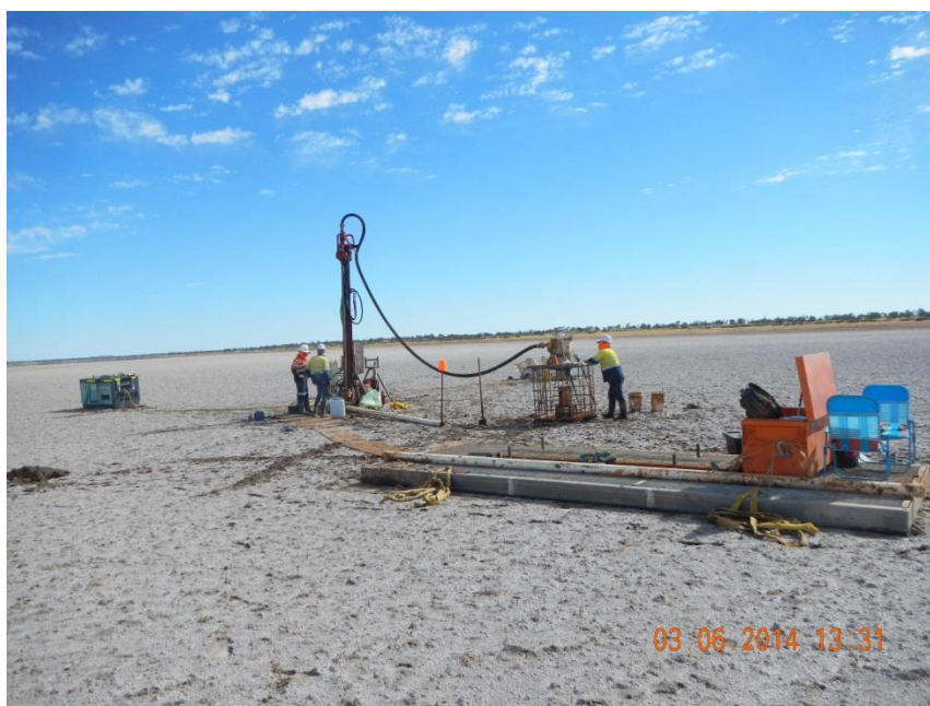
Figure 1. Heli-portable air core drill rig on Lake Hopkins.
