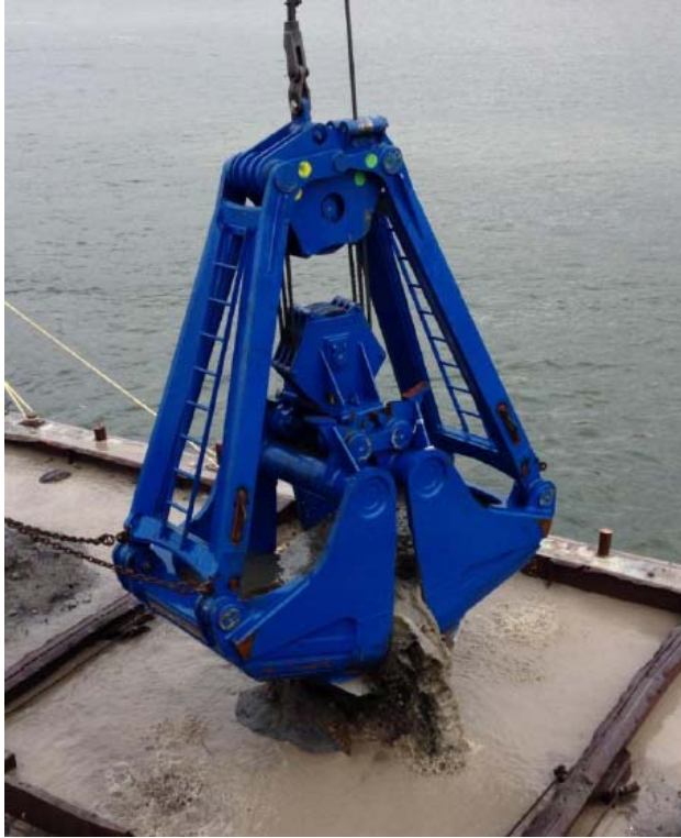
Figure 1 – Example of a mechanical clamshell grab (image courtesy of The Grab Specialists B.V.)
