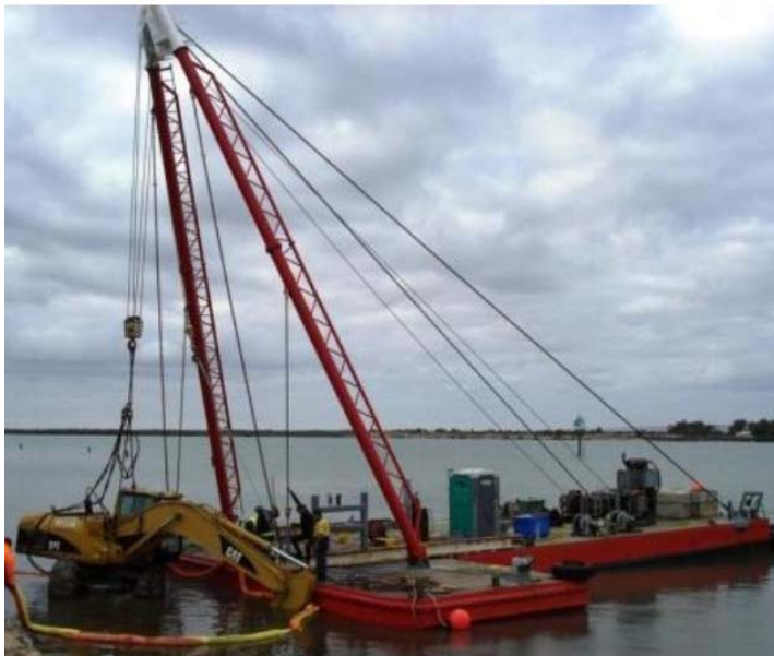
Figure 2 – Example of a shear leg crane on a barge (image courtesy of Maritime Constructions Pty Ltd)
