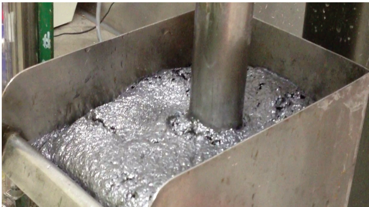
Figure 1- Graphite Concentrate in the Laboratory Flotation Cell
