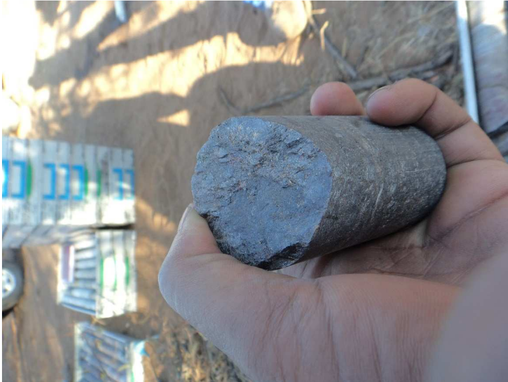
Picture 2: sample of the diamond drill core intercepting graphite.
