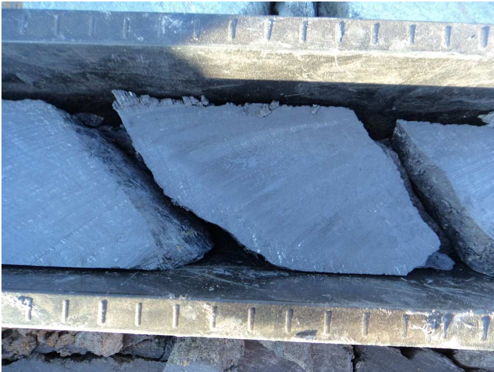
Picture 1: shows graphite in the diamond core cut for preparation for laboratory analysis.
