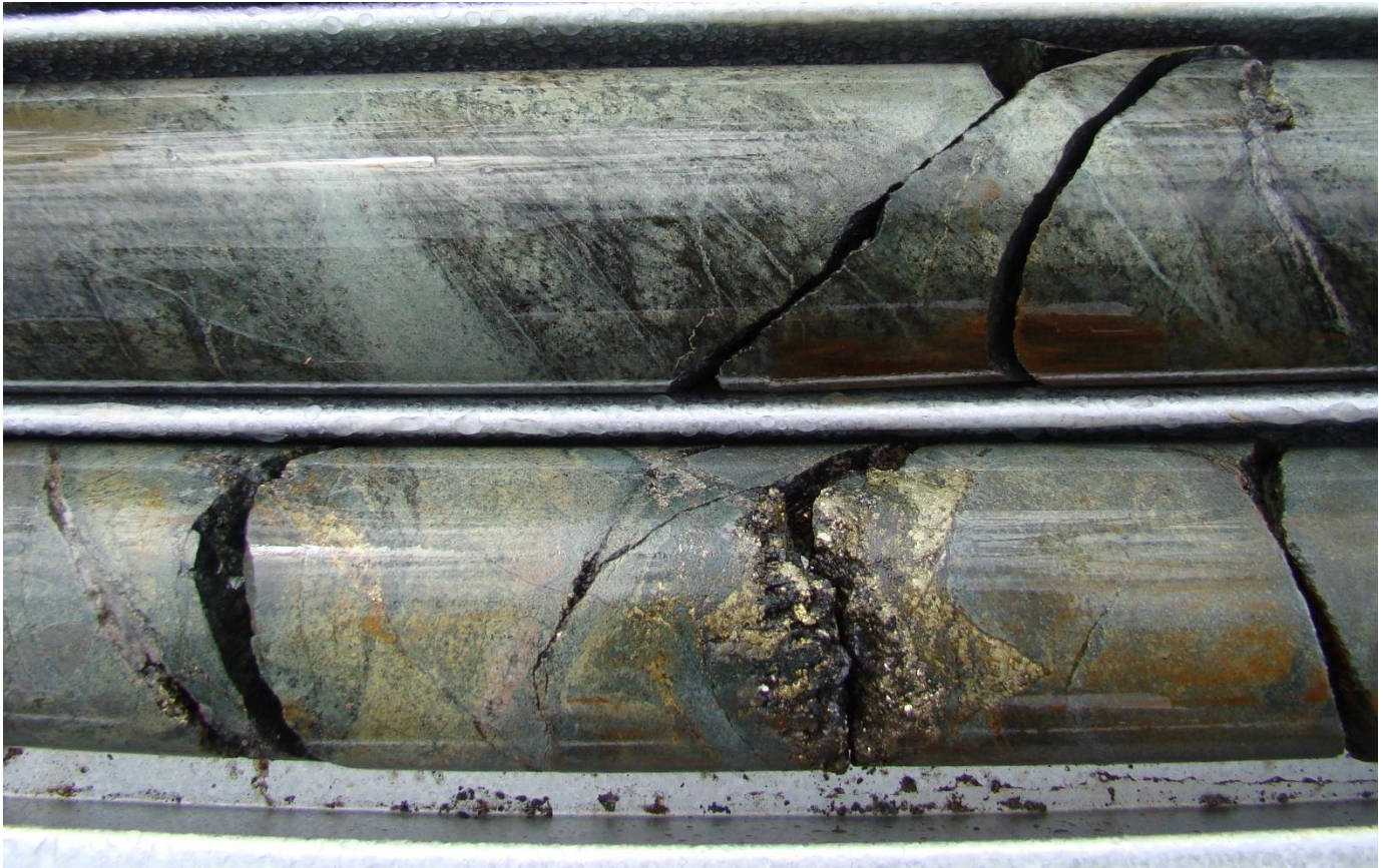
Photo 4. Chalcocite, chalcopyrite, and pyrite in pillow margin
