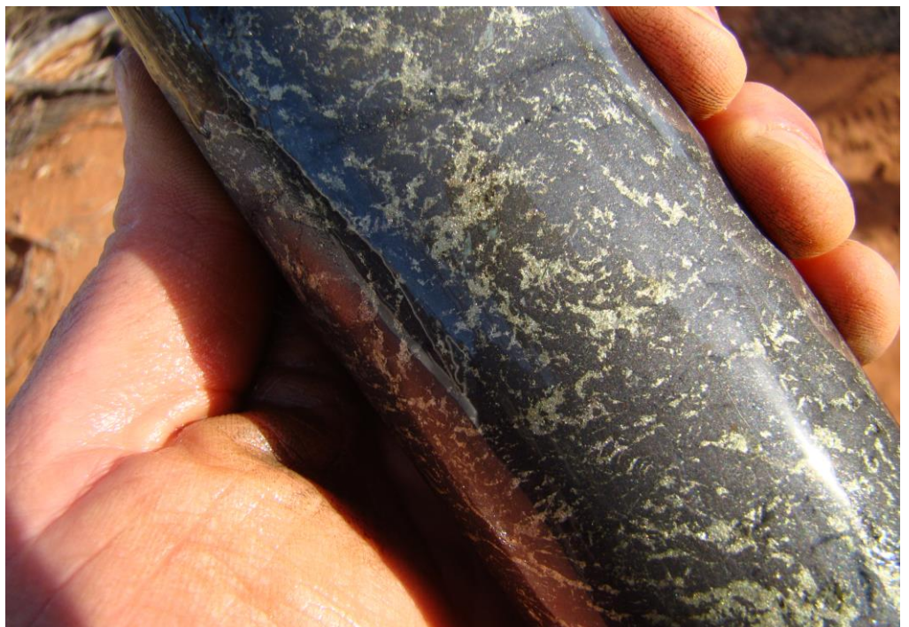
Photo 1. OBUDD001 (257m): Massive magnetite-copper-gold mineralisation
