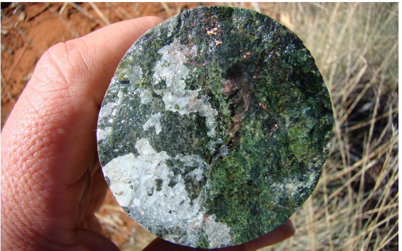
Photo 5. Native copper on joint surface
