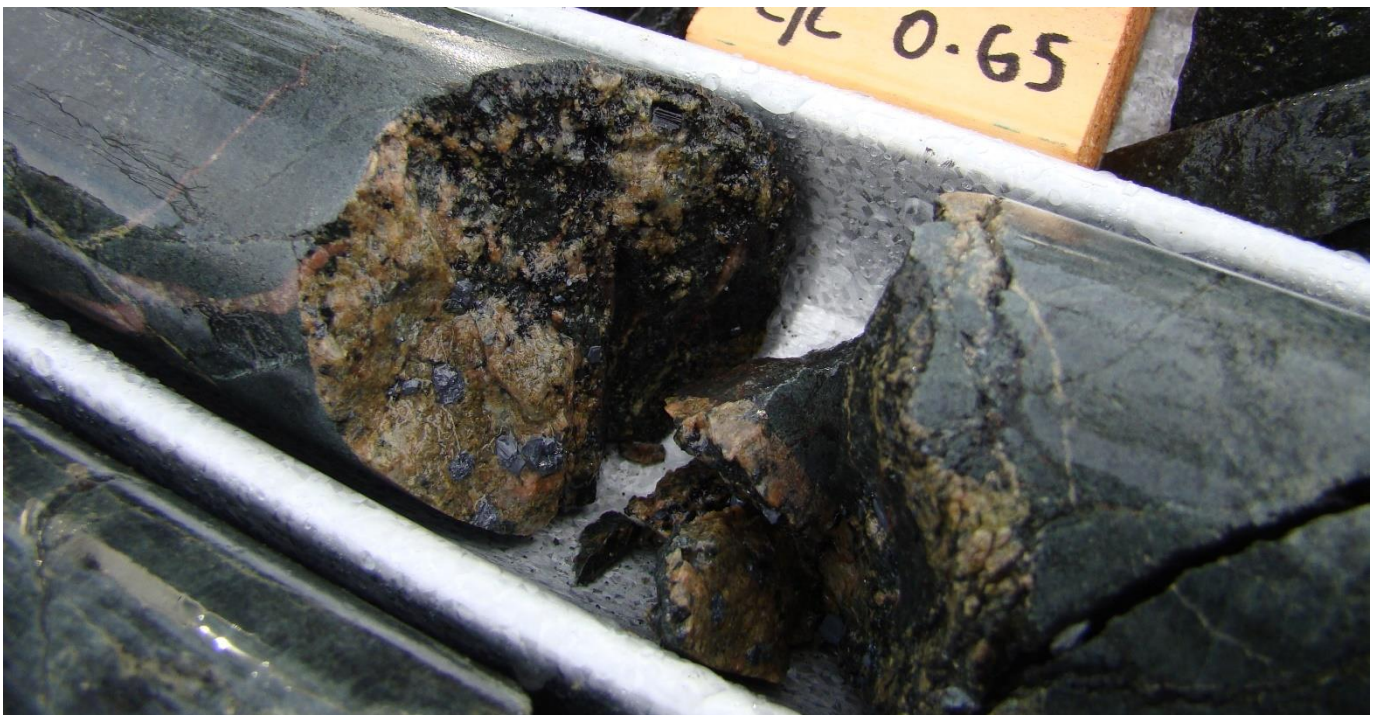
Photo 3. Secondary chalcocite on joint surface
