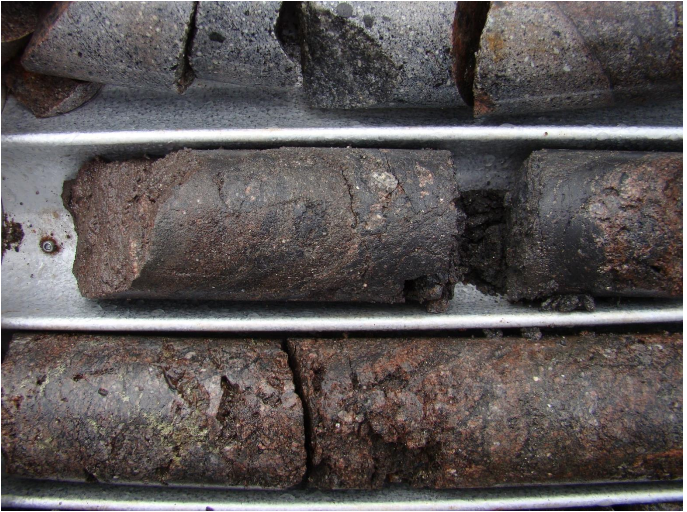
Photo 6. Degraded intermediate intrusive with chalcocite, chalcopyrite, and pyrite
