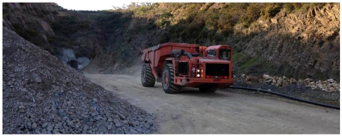
Recently acquired Toro 45D underground truck carting waste rock from the decline. Scalped pile of low grade ore in left of image.
