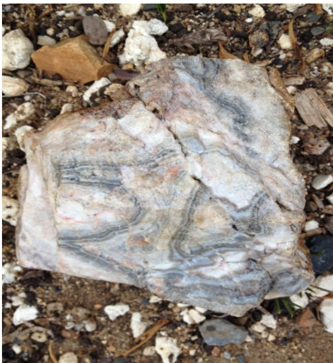
Crustiform-Colloform Quartz with blue chalcedony (left), and banded veins (right) are observed.
