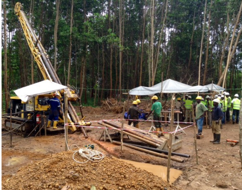
Figures 2 & 3 | Field pictures of diamond drill rig and core taken during a recent Project site visit by the Liberian Ministry of Mines, Land and Energy delegation.
