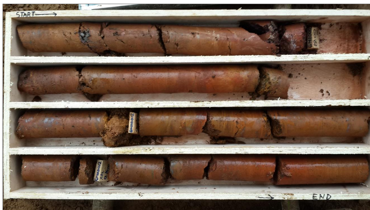
Figure 13 | Diamond drill core recovered from the first drill hole of the PFS programme at the Gofolo Main deposit; high-grade hematite-goethite mineralisation, depth approximately 18-22m down-hole.
