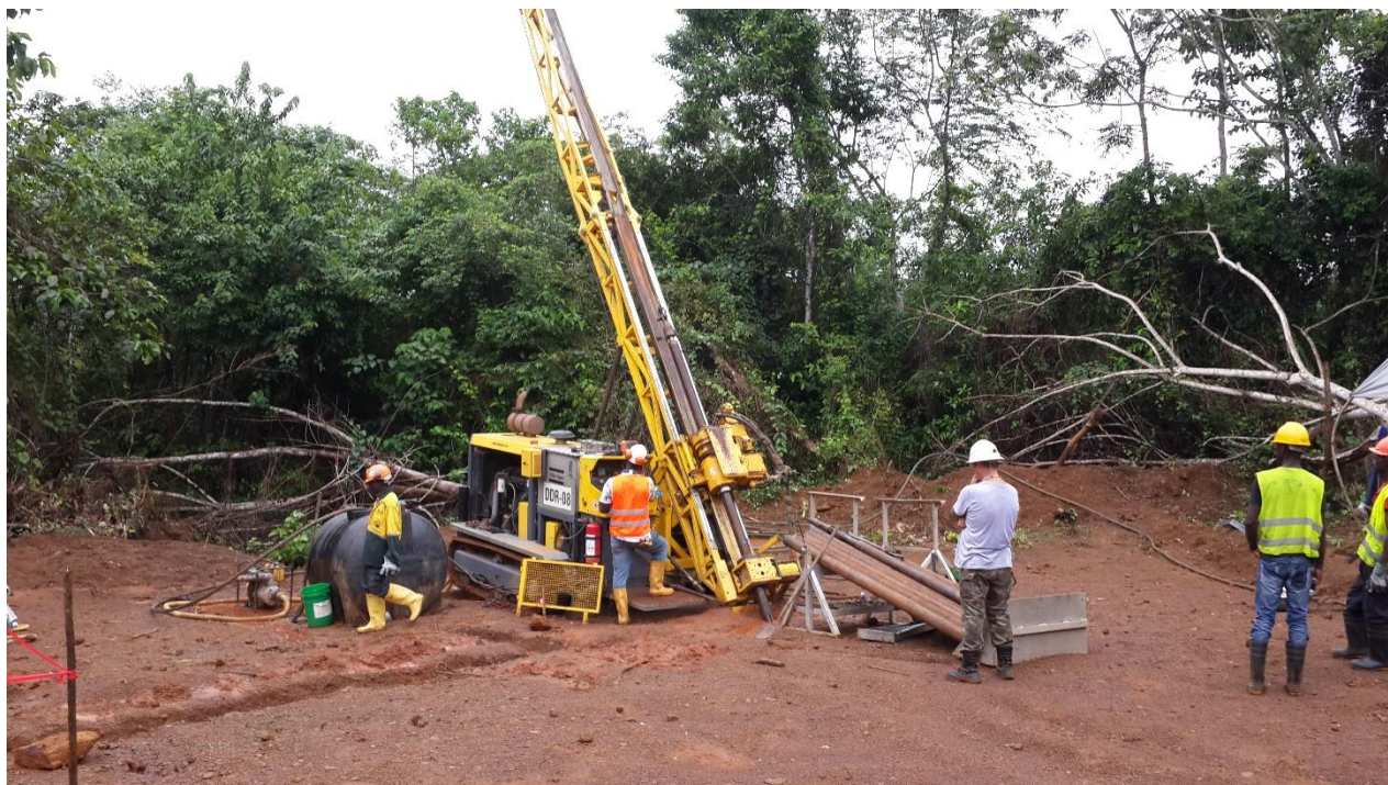
Figure 12 | Diamond drilling carried out at the project site in August.
