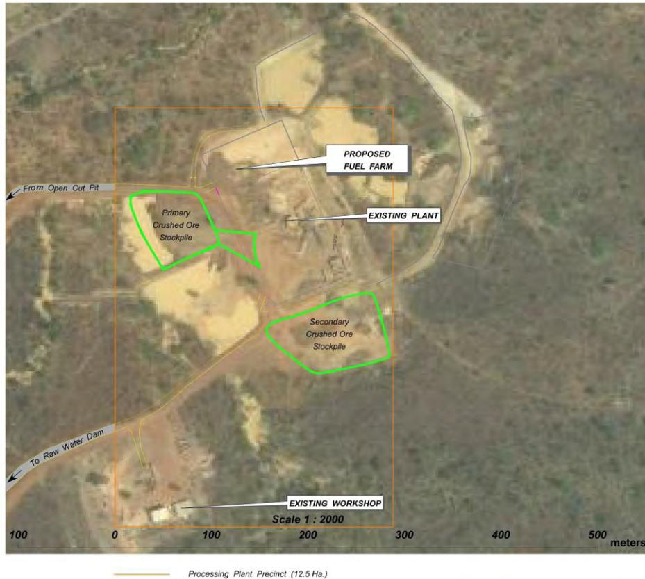
**Figure 2 – Processing Plant Footprint**
