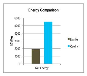
In the case of Victorian lignite, Coldry delivers an 80% reduction in moisture content and an increase of around 280% in net calorific value (wet basis).
