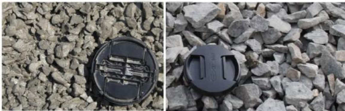
Figure 16-18: Unscreened stemming before (left), screened stemming after (right)
