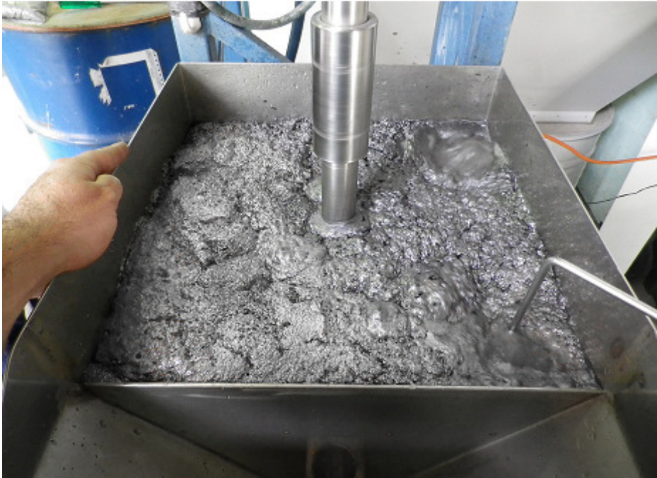
Figure 2: Larger Scale (60L) Flotation Test
