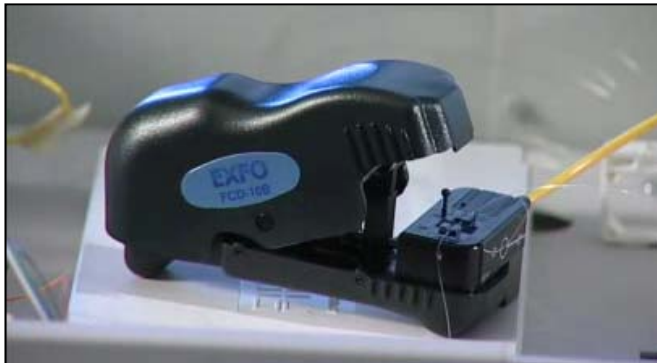
Inexpensive, easily accessible hacker's clip-on coupler device
