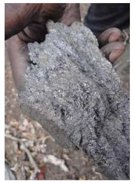
Figure 12(b): Coarse flake graphite in a sample from NTR002. Historical metallurgical testwork (Van Eck & Lurie – Batepro Labs) shows that simple flotation can produce a concentrate grade of 98.3% carbon.
