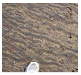
Figure 7(b): At the Tongani Prospect, extensive mineralisation outcrops with a valuable assemblage dominated by ilmenite with 7-10% rutile and 4-6% zircon. The extensive hand auger drill programme that has been conducted over the past year was guided by outcropping mineralisation as well as high resolution aeromagnetics and radiometrics conducted in 2012.
