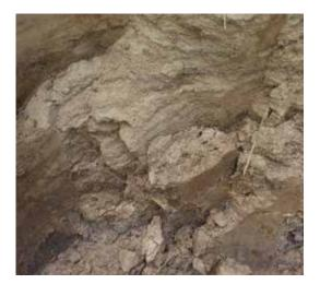
Figure 6(b): Mineralisation from most southerly sample location showing bedded mineral sands (estimated at 10-15% HM) in a small cliff outcrop.
