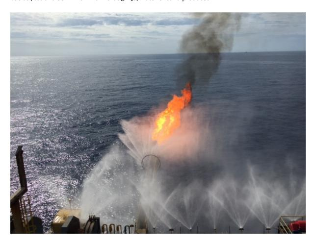
DST-1 was conducted in the Maastrichtian B sandstone reservoir over the interval 1,926-1,953 mRT. The maximum oil flow rate attained was 3,360 stb/d (stabilised rate of 2,300 stb/d) through a 44/64" choke with a flowing tubing head pressure of 690 psia and a gas-oil-ratio of 620 scf/stb. At the end of the main 36 hour flow period, the well was shut-in for a 57 hour pressure build-up period.
