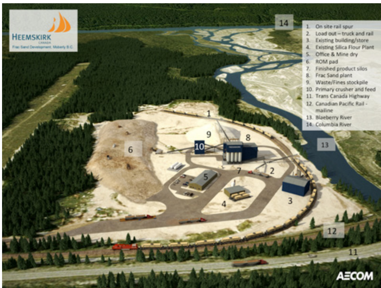
FIGURE 2: LAYOUT OF PROPOSED PLANT AT EXISTING MOBERLY PLANT SITE
