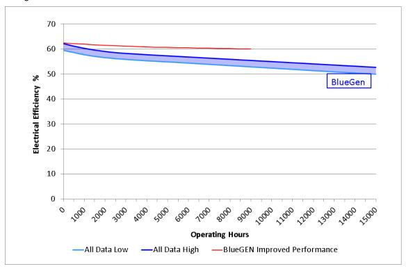
This stack is now in its linear phase of degradation and this data has been extrapolated to show the expected life to reach the same efficiency as the blue shaded section in the above graph. This extrapolation indicates a stack life of approximately 60,000 hours or close to 7 years.
