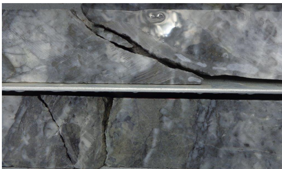
Figure 3. Epithermal veining with alteration and disseminated sulphides, hole AFRCD004.
