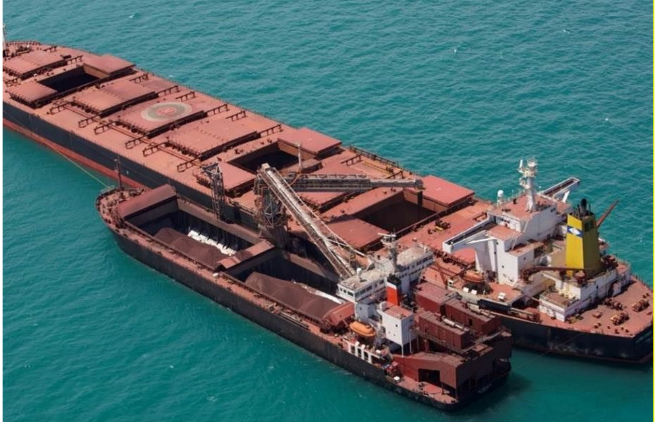
Figure 6 | Self-unloading TSV, directly into an Ocean Going Vessel (OGV).
