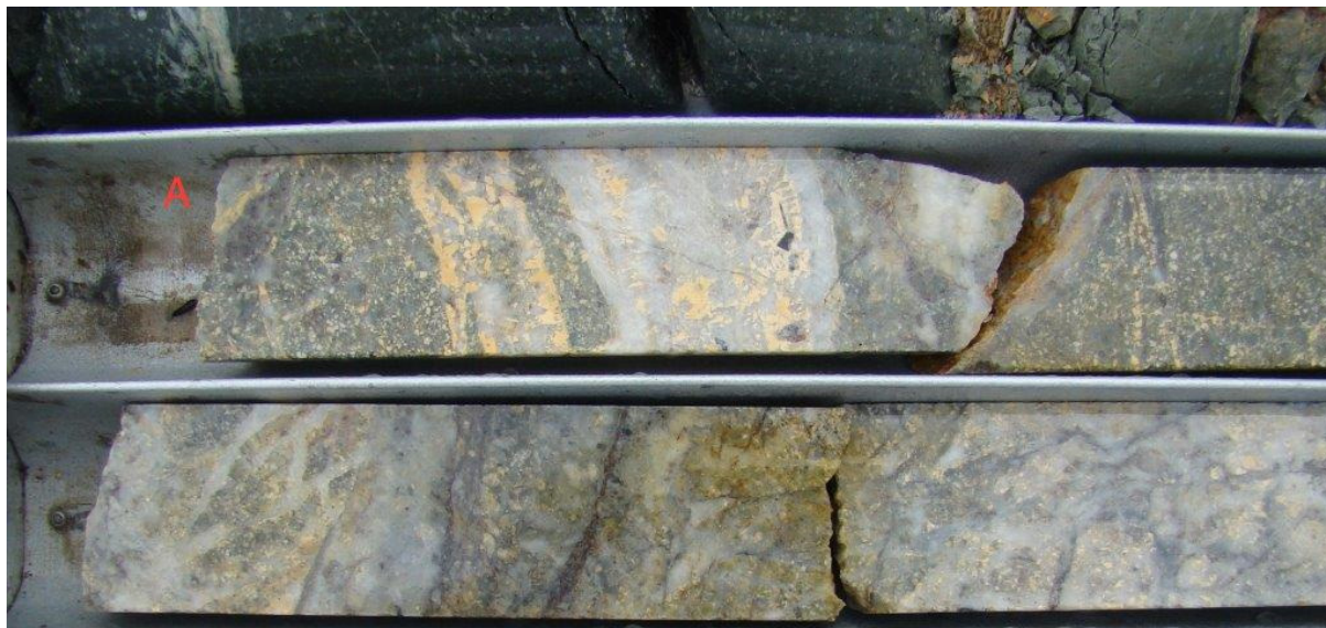
Figure 7: Strong cream coloured adularia deposition with epithermal textured quartz vein. VGRCD2 depth 94 metres.
