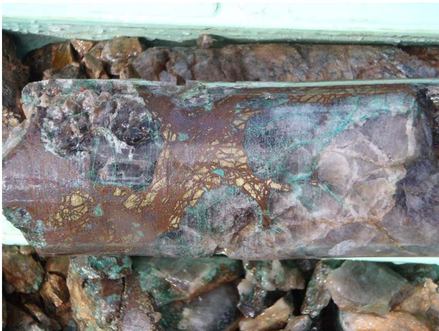
Figure 1 Section of core from GTD002 showing copper mineralisation including chalcopyrite (yellow), bornite (brown) and malachite (green) within quartz veins
