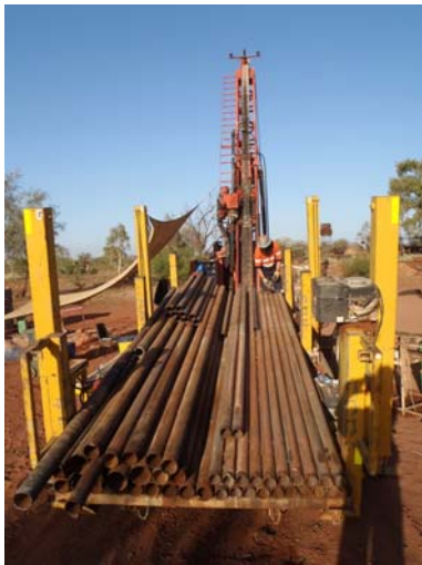
Figure 2 Diamond core rig currently drilling at Marshall-Reward Deposit.
