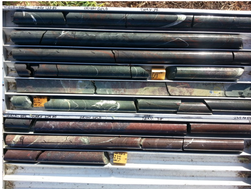
Figure 3: Drill core intersection of a broad zone of strong haematite alteration, potentially related to a proximal porphyry intrusive. Drillhole VGRCD002.
