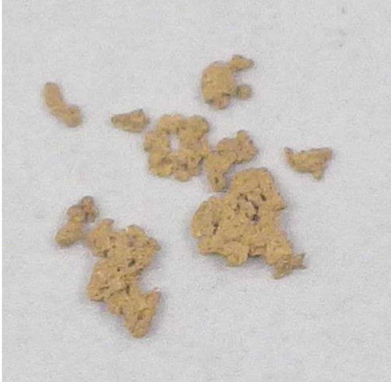
Figure 3: Gold recovered (0.00995g from 39.24g sample)
