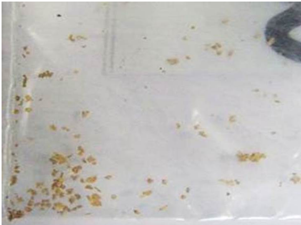
Figure 2: Gold recovered (0.02g from 200g sample)
