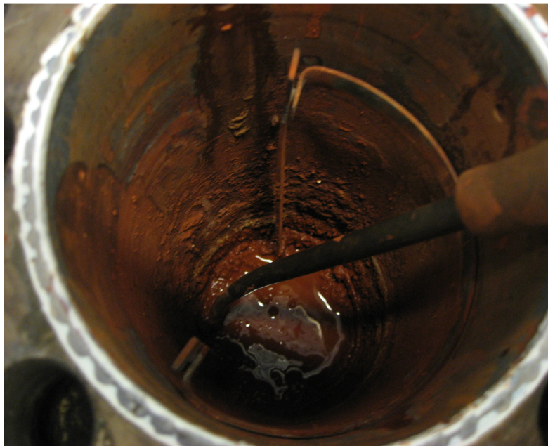
Figure 3. Caking and crust formation on the walls of autoclave
