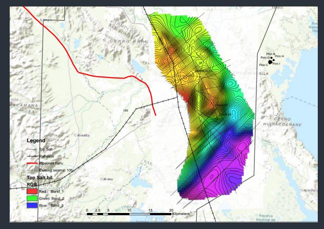
Contour interval is 20 ms or ~40 m in vertical relief
