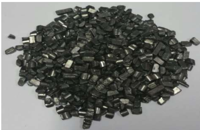
Figure 3 – Trial Balama graphite recarburiser briquettes
