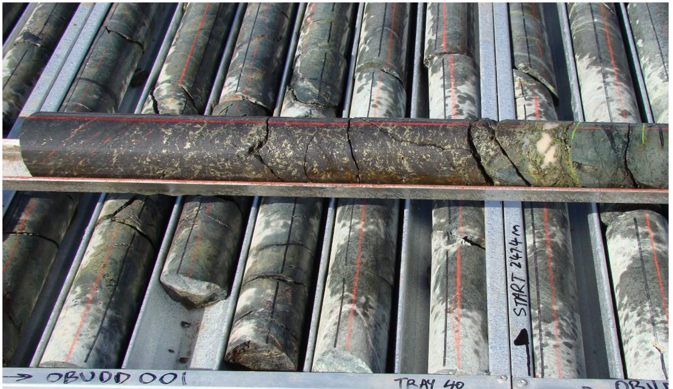
Photo 1. OBUDD001: Massive magnetite-chalcopyrite at base of feeder structure (0.9 metres @ 4.5 g/t Au & 2.6 % Cu from 256.4 metres depth)
